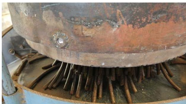
Pellets being produced under high pressure.
