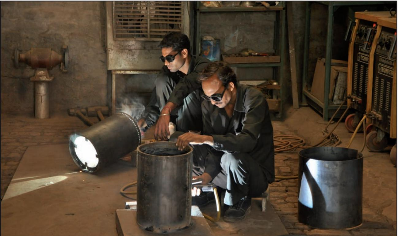
Construction of combustion chambers: The efficient cookers project replaces polluting liquefied petroleum gas (LPG) cookers with climate-friendly biomass cookers.
