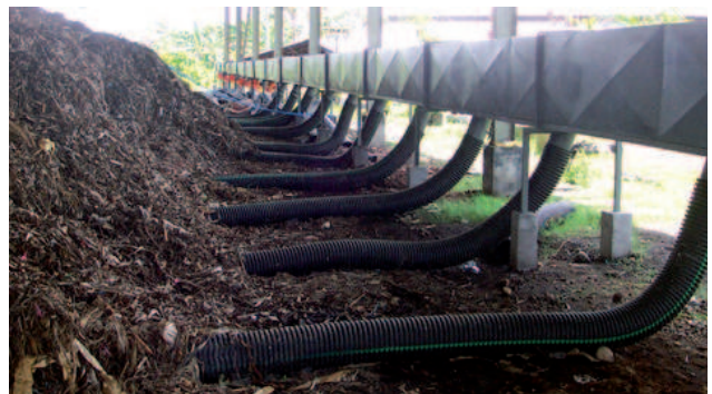
To ensure aerobic decomposition, air is pumped into the compost material.
