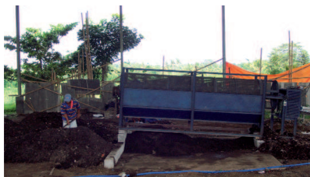
New compost sieve: non-conical, self-cleaning and long-living.
