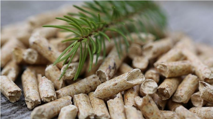
The cylindrical wood pellets are up to 4 centimetres long and have a diameter of 0.6 centimetres. Photo: [www.proPellets.ch](http://www.proPellets.ch)
