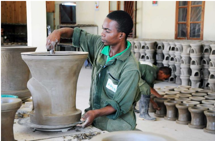
Benjamin Rakotovaomanana on completion of a clay combustion chamber for schools. Photo: Angela Zimmermann
