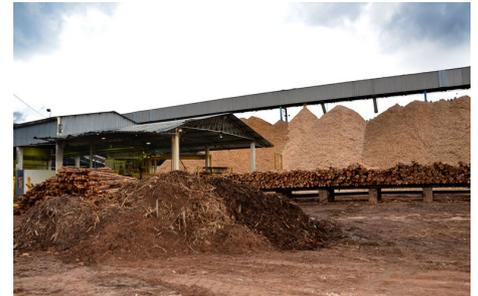
Stockpiled sawdust (in the back) and wood logs ready to be chipped and mixed with the biomass residues in order to be fed into the biomass boiler.
