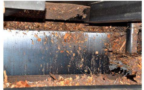
Entry point of mixed biomass into the biomass boiler.
