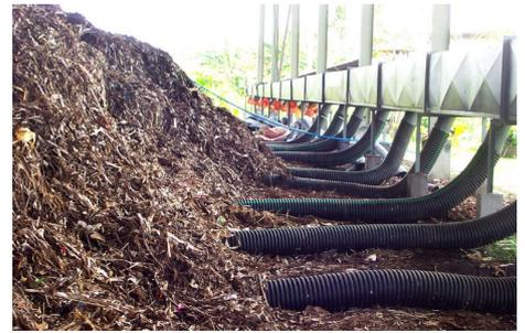
The biomass is aerated to ensure aerobic composting, resulting in the production of carbon dioxide and heat rather than methane.
