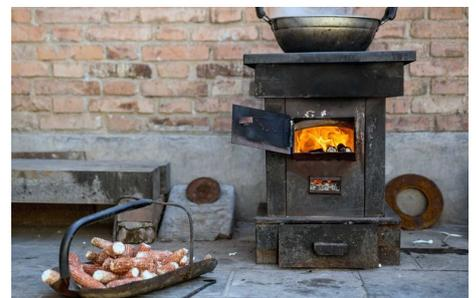
The new efficient stoves can be lit with the rest of the corn cobs, which were not being used before the project.
