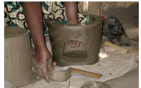
Efficient stoves are manufactured using standardized tools to guarantee stove's quality and efficiency.
